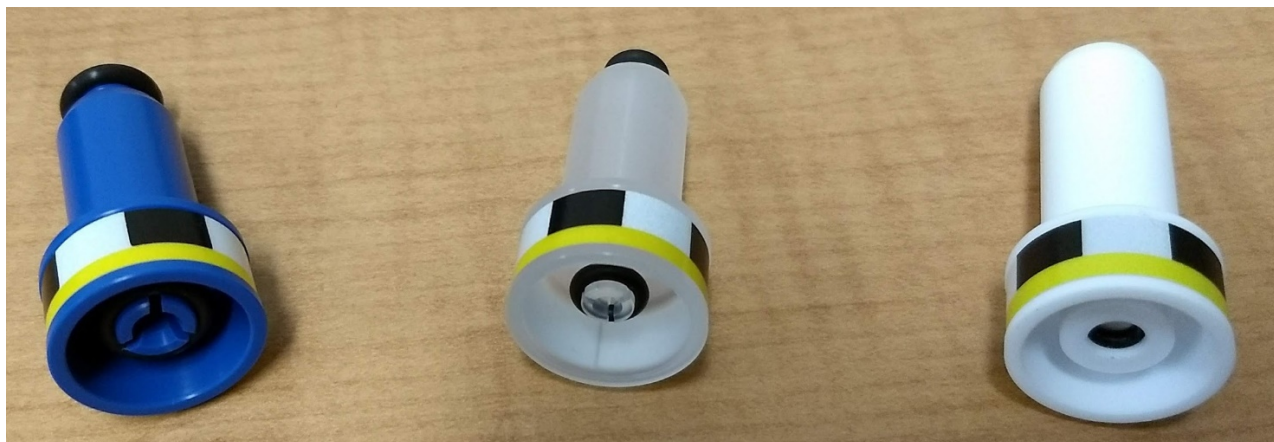
Fig 1: Three types of spinners: Standard POM Spinner (blue, left), 0°C to +80°C; Kel-F Spinner (off white, middle) for elevated Temperatures, +80°C to +120°C; Ceramics Spinner (white, right) for high and low Temperatures, +120°C to +180°C and 0°C to -150°C (A600, Au400, and Hg400)
